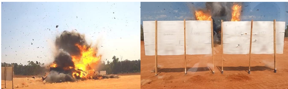
Fig. 1. Detonation of a VBIED (image courtesy of RUREX Pty. Ltd.), and fragments impacting a witness panel.
