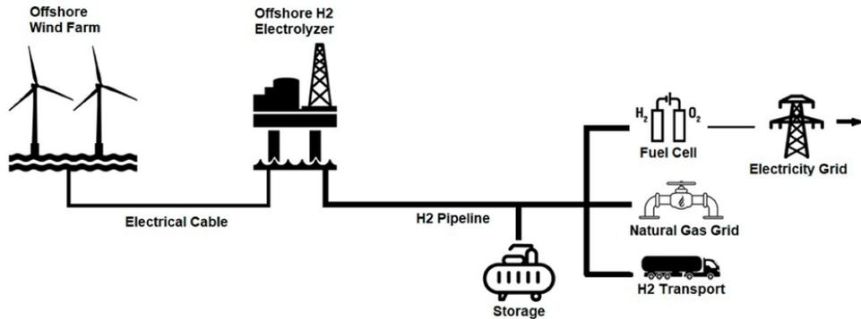
Fig. 3. Hydrogen production within an offshore platform (Calado and Castro, 2021).
