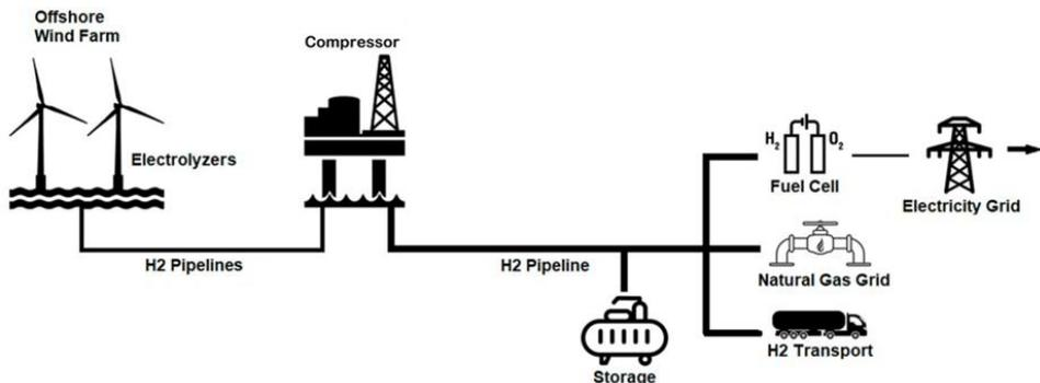
Fig. 2. Hydrogen production in individual wind turbines within OWF, with centralized compressor, modified from (Calado and Castro, 2021).
