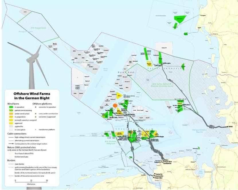
Fig. 4. Existing and planned OWFs in the German North Sea EEZ (Dörrbecker, 2020). The operating OWFs are marked with green and the planned ones with yellow and grey colors. The area chosen for our case study is marked with an orange circle.
