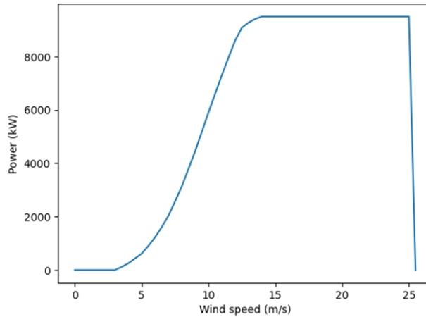
Fig. 5. Power curve of the VESTAS V164-9.5MW (The Wind Power, 2023).
