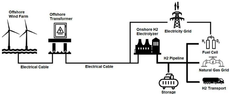
Fig. 1. Onshore hydrogen production with electricity produced in OWF (Calado and Castro, 2021).
