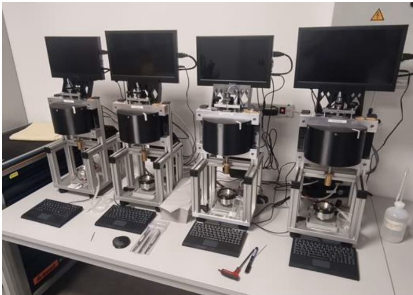
Fig. 5. Newly developed test rig for fatigue tests of dental implants to ensure the long term reliability: Four fully assembled versions in the laboratory.
