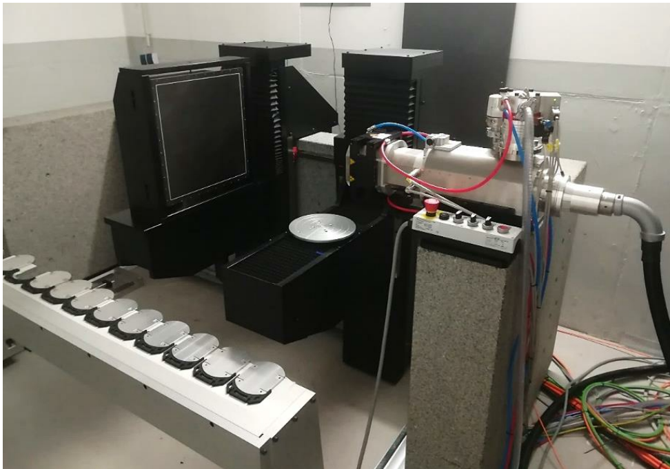
Fig. 3. Used \mu -CT system with transmission X-ray source and flat-panel detector (Source: diondo GmbH).
