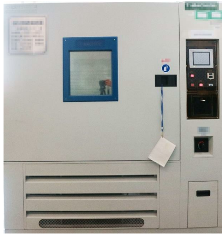
Fig. 3. The constant temperature test chamber used in this test.
