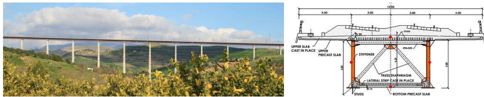
Fig. 3. Elevation view of the monitored viaduct “Arroyo las Piedras” and its cross-section (Cornejo, 2010).
