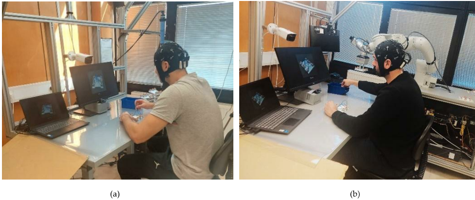
Fig. 1. (a) Standard Scenario (SS): the assembly task is performed by the participant without any external intervention in the workplace; (b) Collaborative Scenario (CS): the assembly task is performed by the participant interacting with the robot in the workplace.
