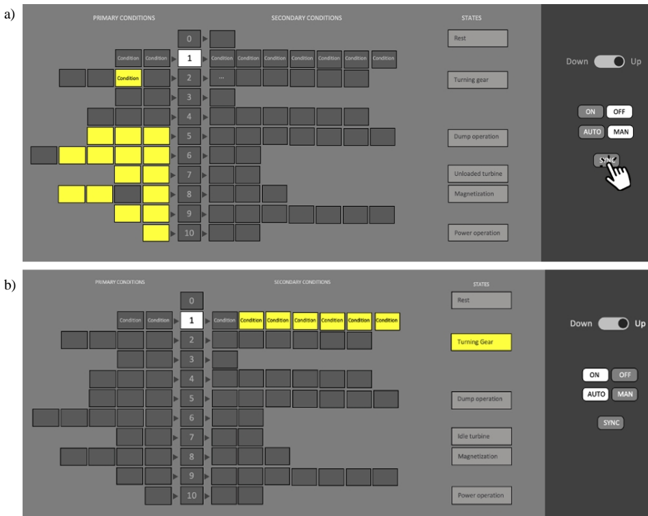
Fig. 1. Principle sketch of the Turbomat interface. When it runs up the turbine it works sequentially from top left to bottom right.
