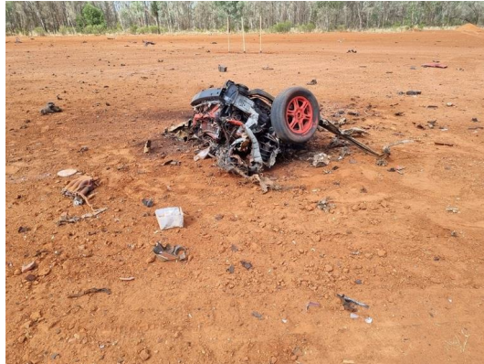
Fig. 5. Photo of body of red vehicle and its location with respect to the blast gauge (3 m to the left of the car body).
