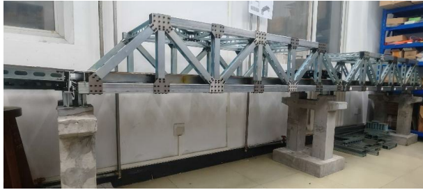
Fig. 4. Experimental truss bridge.
